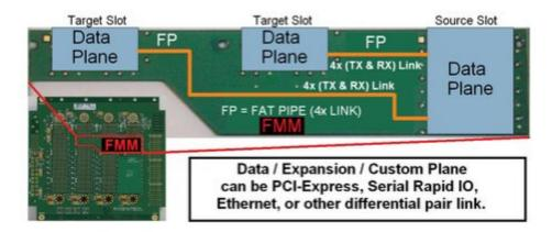
Figure 1: Expansion diagram of FMM micro overlay with two fat pipe PCI Express links (click graphic to zoom by 1.9x)
